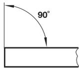
1. Ensure that the end of the tube is cut square and is free from burrs.
